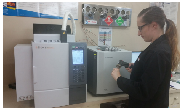
Convex Laboratory Technician Courtney-Ruth Gill operating the new GC machine, which checks that any retained printing solvents in film are within regulated safe levels for food packaging.
